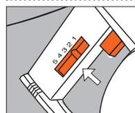
3. Adjust orange rate adjuster to correct setting based on the product being applied. (See chart at right)
