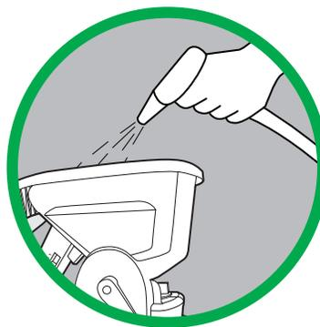
**Clean spreader after use** to maintain proper operation. Perform cleaning over lawn. Do not allow product and /or rinse water to enter storm drains or sewers.
